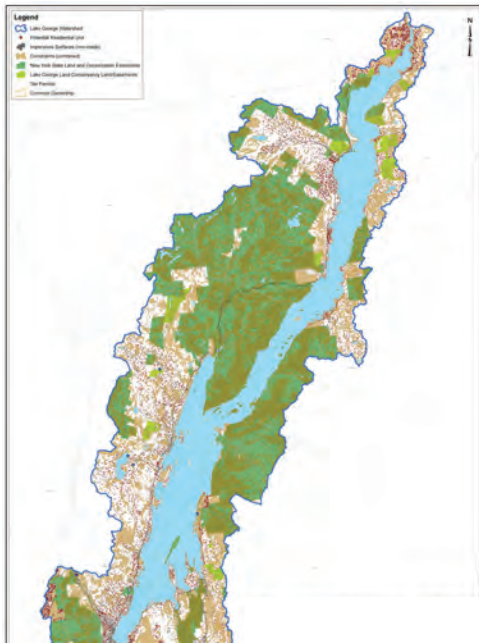
A sample watershed map, demonstrating residential buildout potential, environmental constraints, and existing impervious surfaces within the Lake George watershed
